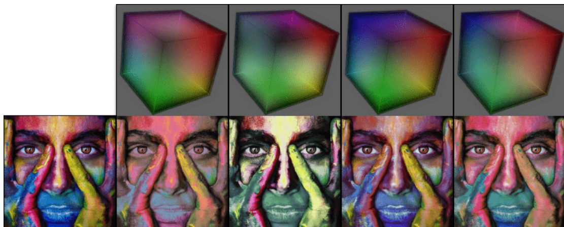
Fig. 3.1.2. Multiple randomized 3D color LUTs obtained via the random_clut command, and applied to a color image.
