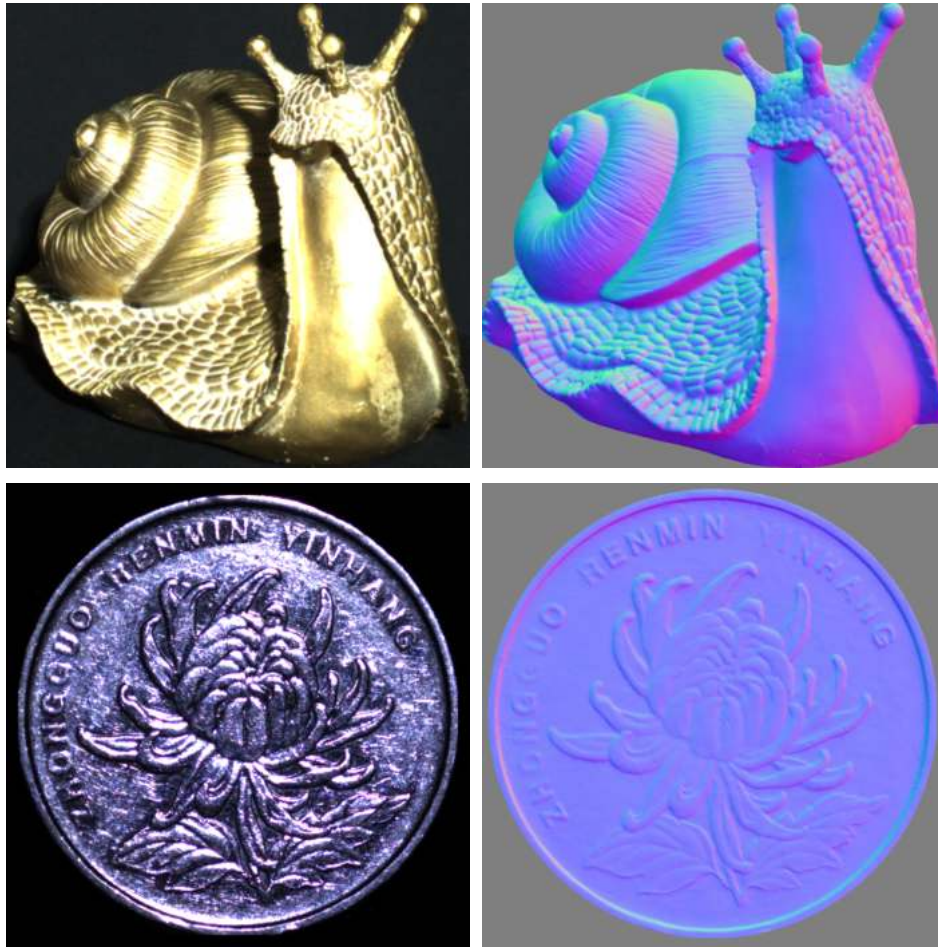
Figure 2: Reconstruction of a normal map of a snail from [38] and a coin from [39] by photometric stereo with our proposed method. We can see that our method manages very difficult materials such as metal.
