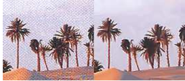
(b) Removing pattern noise from a 555 \times 367 color image. (detail, 1 iteration, processing time: 11 seconds)
