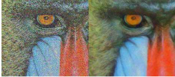
(a) Removing grain noise from a 512 \times 512 color image. (detail, 1 iteration, processing time : 19 seconds)
