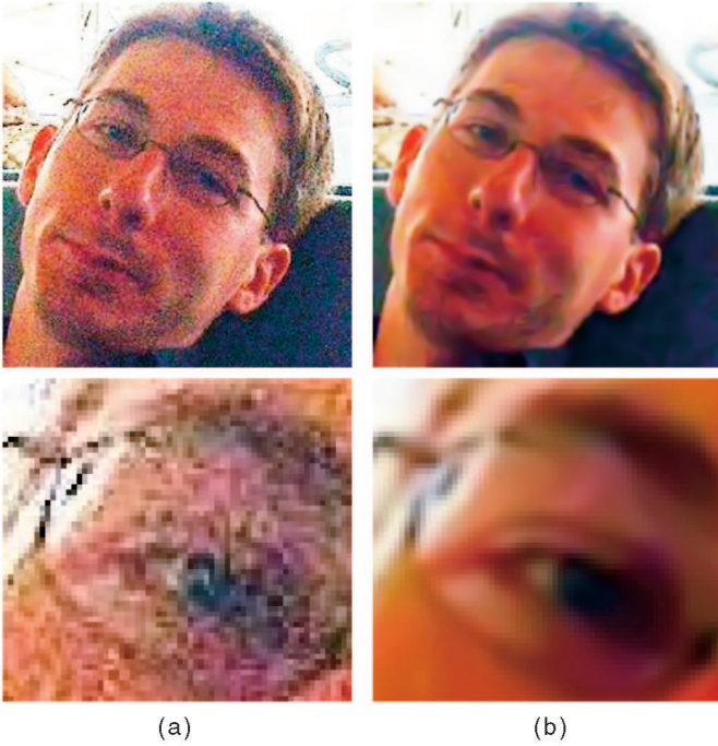
Fig. 8. Using our vector-valued regularization PDE (14), for color image restoration. (a) Noisy color image and (b) restored color image.
