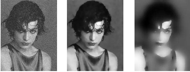
(a) Original noisy image (b) \frac{\partial I}{\partial t} = \text{div}(\mathbf{D}\nabla I) . (c) \frac{\partial I}{\partial t} = \text{trace}(\mathbf{D}\mathbf{H}) .
